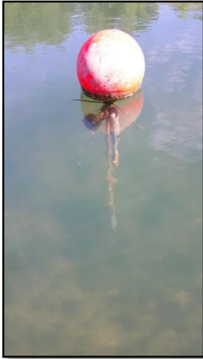
Conductivity and temperature probes installed in the top and bottom of a pond
