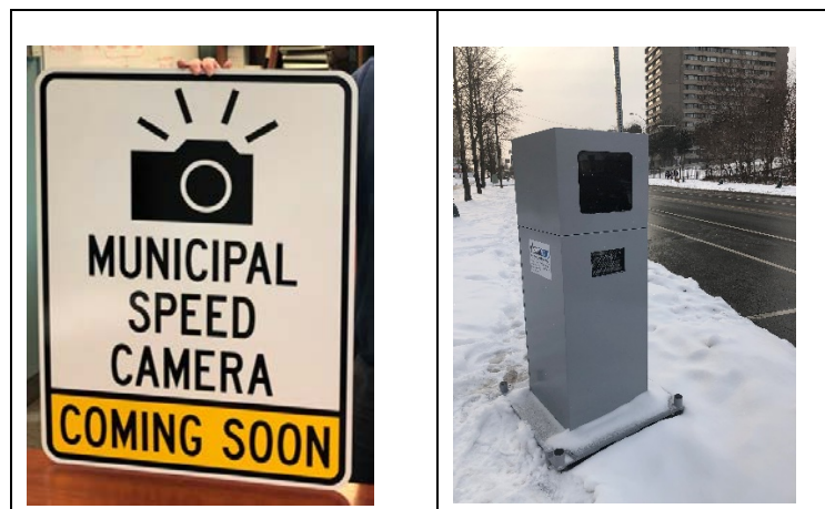
Figure 1: Advance Warning Sign and Camera Unit
