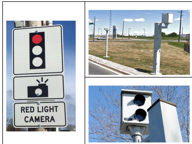
Figure 2: Advance Warning Sign and Camera Unit
