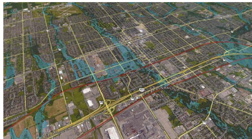
▲ Flooding on Corbett, Oshawa and Harmony Creeks, as a result of “pinch-points” (Central Lake Ontario Conservation Authority).
