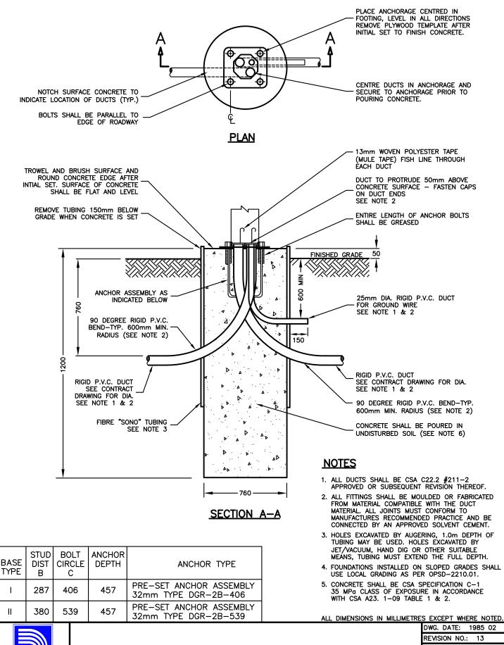
CONCRETE FOOTING FOR PEDESTAL SUPPLY CONTROL CABINET
