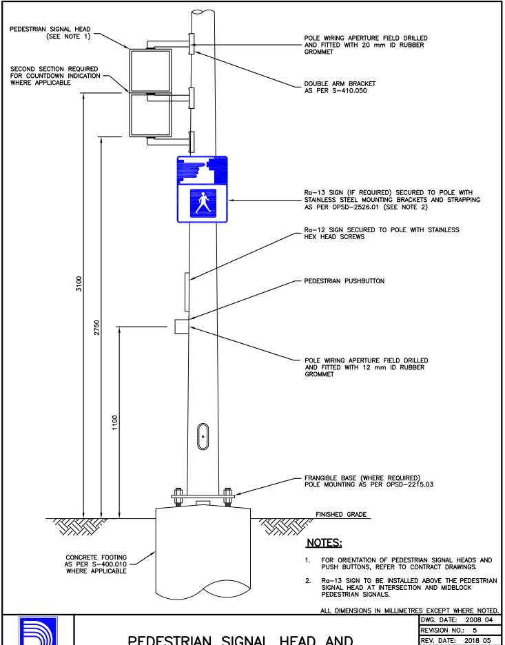
PEDESTRIAN SIGNAL HEAD AND PUSHBUTTON INSTALLATION ON STEEL POLE
